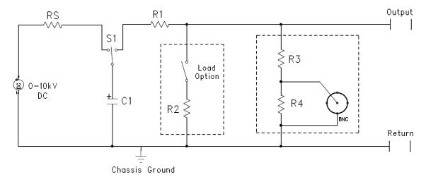
Figure 1. General Diagram Megapulse Antenna Surge PF
