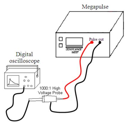
Figure 4. Waveform Measurement Setup
